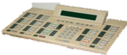
Gambar 2.2 Private Manual Branch Exchange
