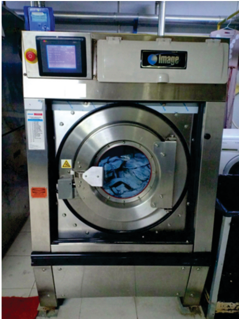
Gambar 3.3. Washing and Extractor machine Sumber: Hotel Eastparc Yogyakarta, 2018
